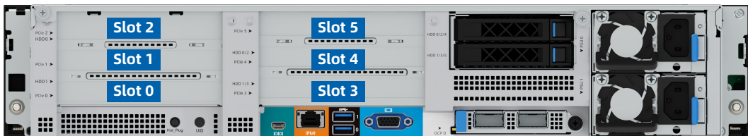
Figure 5-15 PCIe Slots
