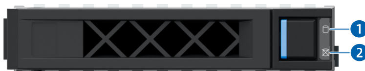
Figure 5-10 SAS/SATA Drive LEDs
