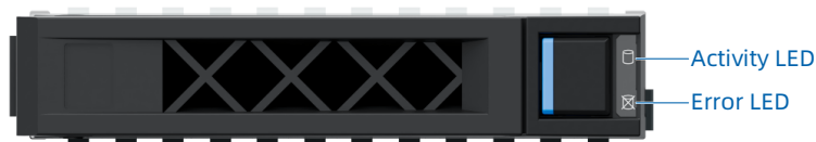
Figure 5-40 SAS/SATA Drive LEDs
