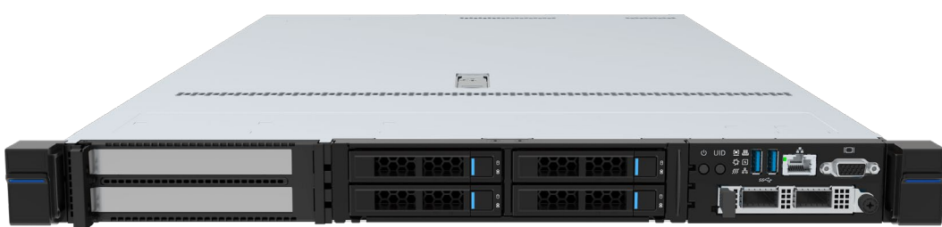
Figure 1-7 4 × 2.5-Inch Drive/E3.S SSD + 2 × PCIe Slot Configuration
