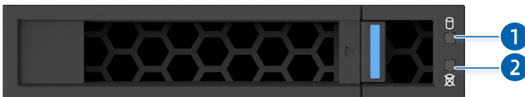
Figure 5-13 NVMe Drive LEDs
