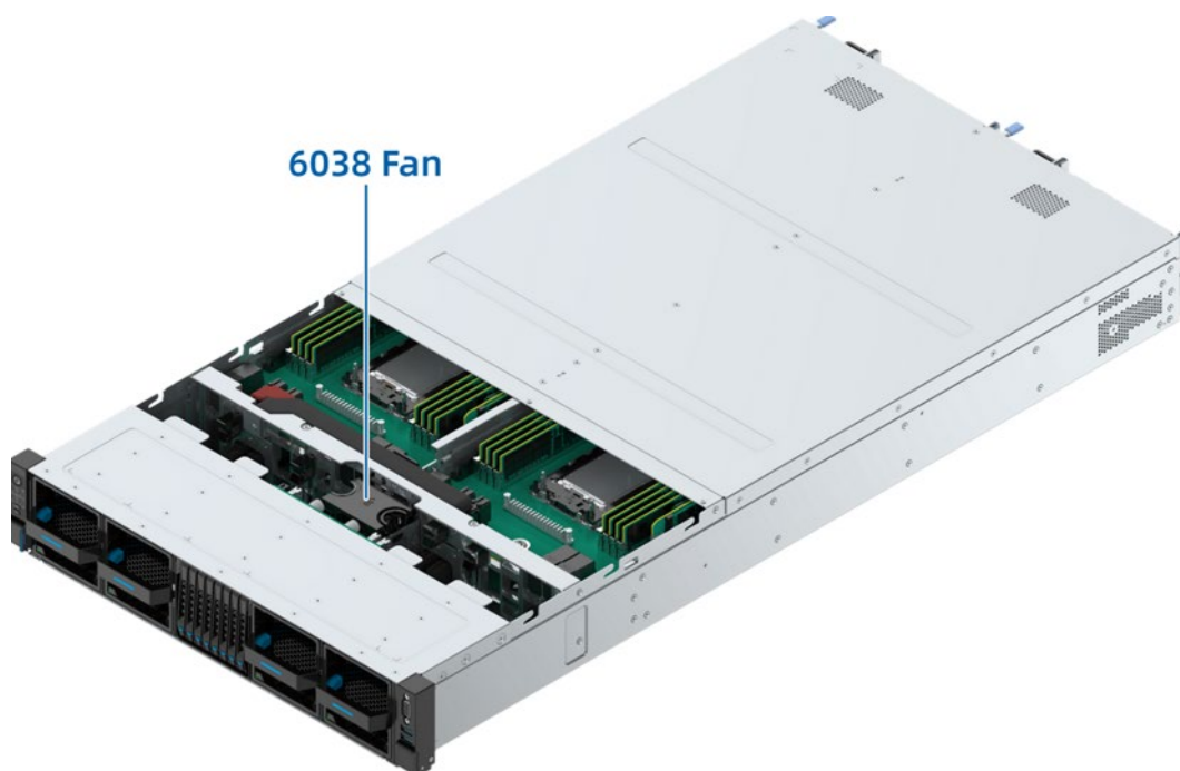
Figure 5-24 Internal Fan Location
