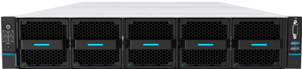
Figure 1-1 K24-E2-A0-R0-00 (5 × 8086 Fan Configuration)
