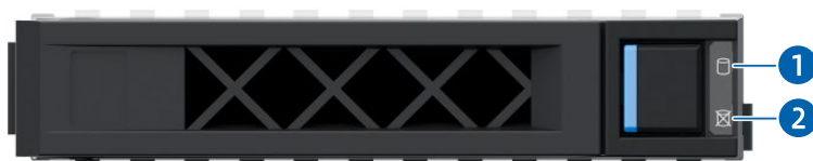
Figure 5-16 SATA Drive LEDs
