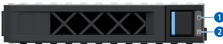
Figure 5-7 SATA Drive LEDs
