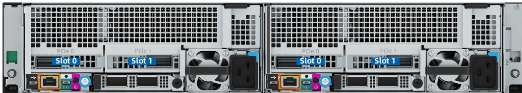
Figure 5-14 PCIe Slot Locations of 4 × PCIe Slot Configuration
